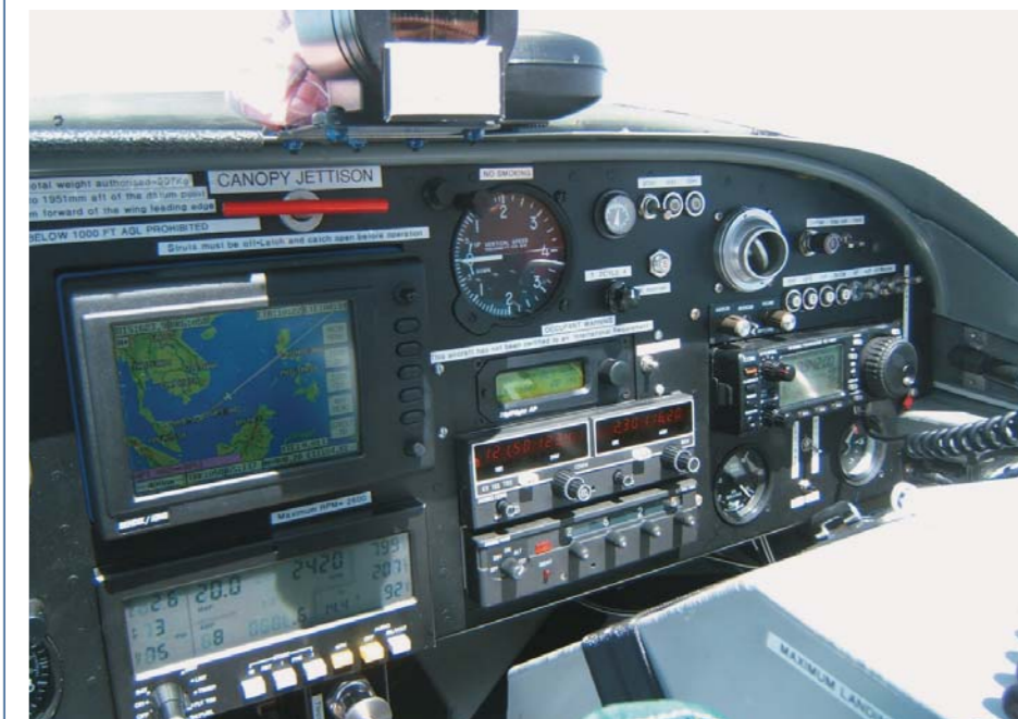
The Bendix SkyMap graphically shows Manuel's track across the South China Sea.
